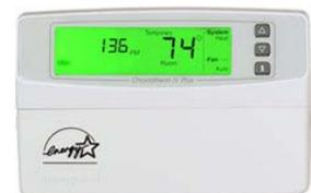
network thermostats allow for even better “zone” control and energy savings. See the [Heating, Cooling & Ventilating](#) section of this Guide for more information.
